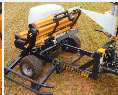
Automatic cut & start system and tip-off
