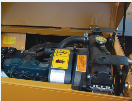
20 hp 3 cylinder Kubota engine allows full operation of the wrapper standard on 1804-S
