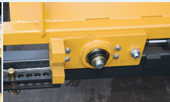
Hydraulically adjustable rollers for quick change of bale sizes
