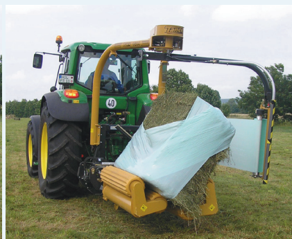
Unique 'Rock & Roll' system rotates bale giving a consistent overlap
