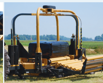
Wrapping process - consistent film overlap for all sizes of bales
