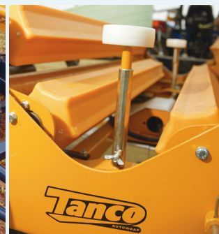
Rock & roll system and bale stop - ensures controlled wrapping
