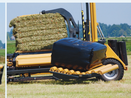
Optional rotate conveyor - allows smooth unload while driving
